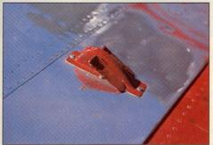
the 35s broke up when flown outside the normal speed/G-loading limits; the vast majority of the break-ups came from the ranks of the oldest airplanes. Amid much controversy and hand-wringing, Beech introduced a fix in the form of tail reinforcements—a leading-edge cuff for some models, with additional stiffeners for others.)
