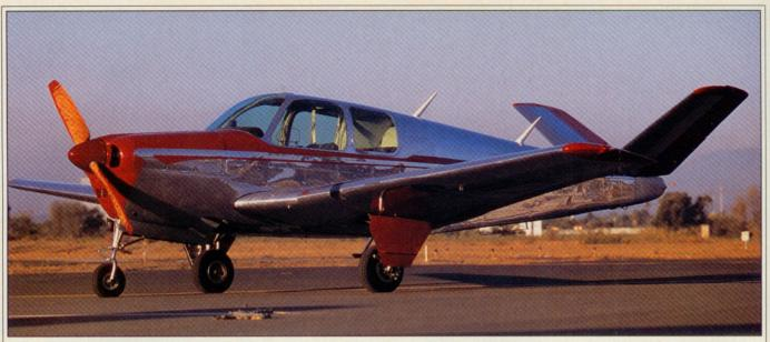
in the S35, the aft bulkhead was pushed rearward 19 inches. While most Bonanza pilots welcomed the additional cabin room, the alteration helped illustrate how the V-tail, once the design's most impressive statement, had come to hinder it. More baggage space spotlighted the restricted center-of-gravity range inherent in the V-tail configuration. Plus, given the fuel tanks' position, the Bonanza's center of gravity moves aft as the trip wears on, further complicating balance considerations.
